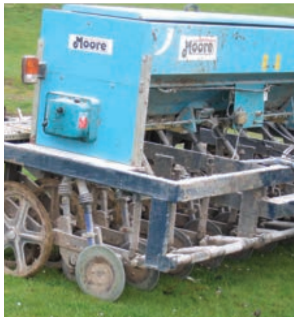
slot seeding into an existing sward
