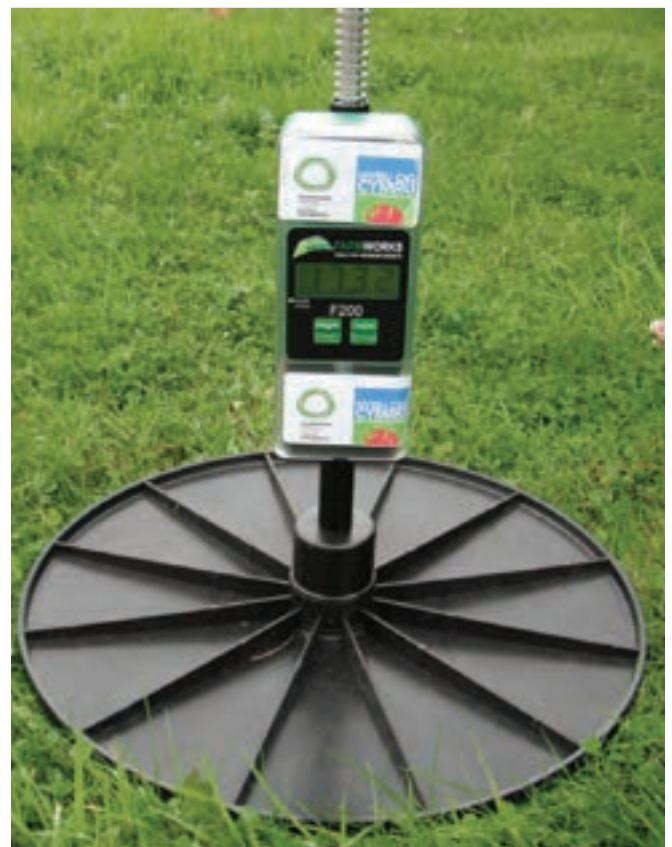
measuring grass with a plate meter
